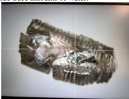
Figure 14. Glass-like carbon crystals found in initial testing at x20 magnification.
