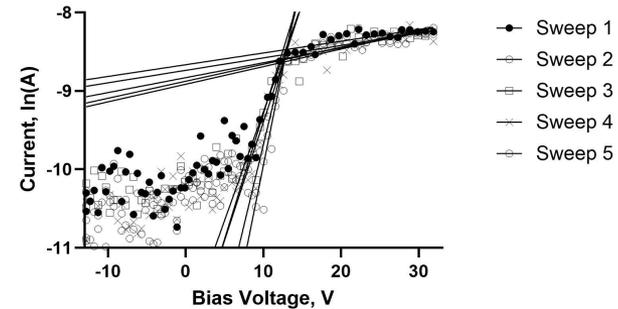
Data from manual method showing a) I-V trace of the probe in ambient plasma and b)  $\ln(I_{\text{probe}} - I_{\text{sat}})$  plotted against bias voltage.
