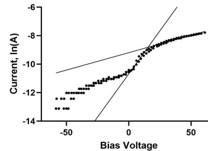
Data from automated method showing a) I-V trace of the probe in ambient plasma and b)  $\ln(I_{\text{probe}} - I_{\text{sat}})$  plotted against bias voltage.
