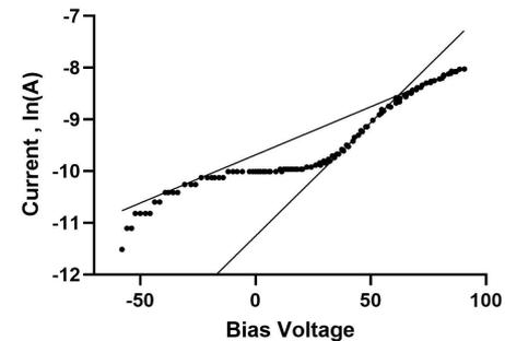
Data from manual method showing a) I-V trace of the probe in adamantane plasma and b)  $\ln(I_{\text{probe}} - I_{\text{sat}})$  plotted against bias voltage.
