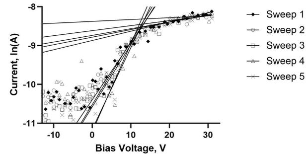
Data from automated method showing a) I-V trace of the probe in adamantane plasma and b)  $\ln(I_{\text{probe}} - I_{\text{sat}})$  plotted against bias voltage.
